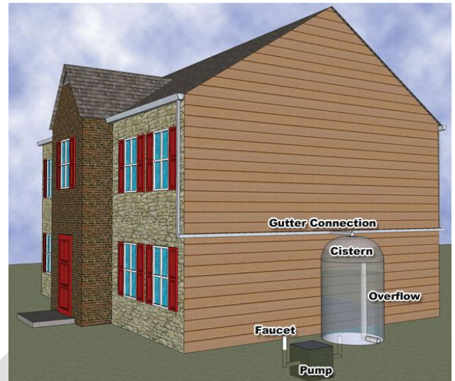
Figure 1: Rainwater Harvesting Components for a Typical, Residential Application (Source: Jones & Hunt, n.d.)
